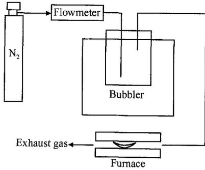
Fig. 1 Experimental setup for oxidation
