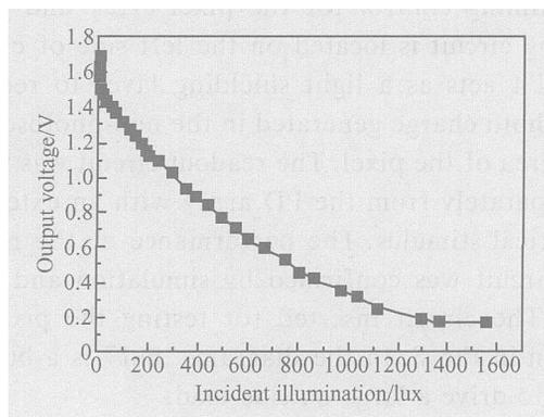
Fig. 5 Output voltage versus incidence density
