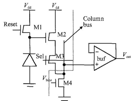
Fig. 3 Test circuit of the pixel
