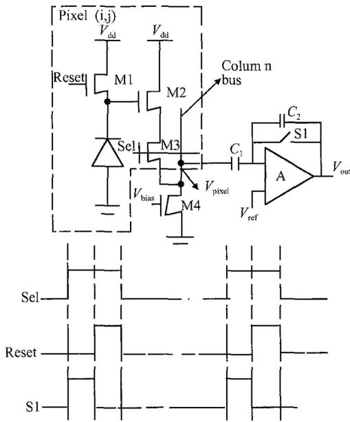
Fig. 1 APS circuit and timing diagram
