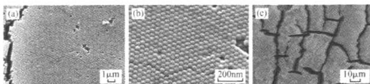
Fig. 2 SEM images of the sample at different plating stages (a) Plating 20s; (b) Magnified pictures of (a); (c) Plating over 200s
