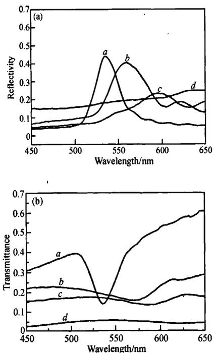
Fig. 1 Normalized optical spectra of the sample at different plating stages at normal incidence (a) Reflection; (b) Transmittance. The electrodepositing times (second) are 0 (*a*), 20 (*b*), 40 (*c*) and over 200s (*d*), respectively.
