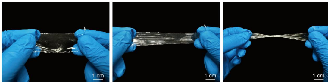
Fig. S2. (Color online) Stretching and torsion of the SEBS substrate.
