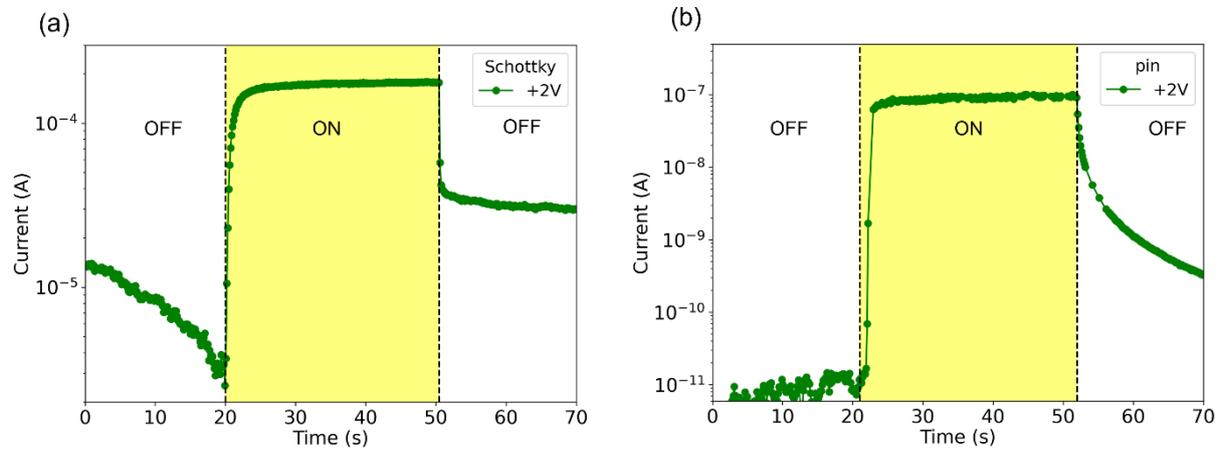
Figure S3: (a) Time response (Current in log scale) for Schottky diode on GaN in positive bias (2V). (b) Time response for pin diode on GaN in positive bias (2V).
