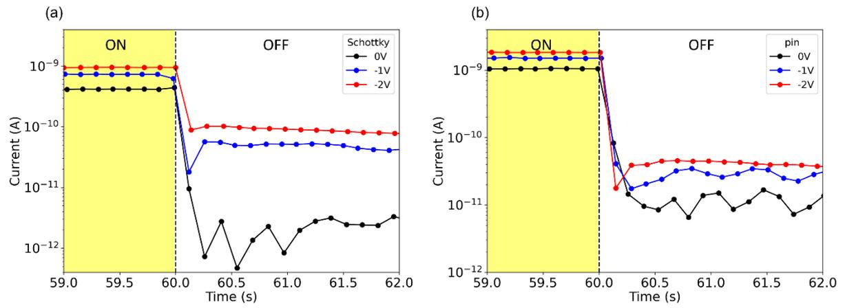
Figure S1: Detail of the time response transient shown in figure 2(c)-(d) for Schottky (a) and pin (b) diodes. The transient ON-OFF is limited by the experimental set-up and corresponds to 150ms.
