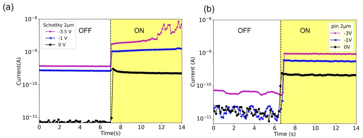
Figure S4: (a-b) Time response of a Schottky and pin diode ((a) and (b) respectively) on sapphire with an active region of  $2\mu\text{m}$ . The response is measured at different biases and represented as a function of time. The beam is initially off and then turned on, the yellow area indicates when the proton beam is turned on ( $132\text{ pA/cm}^2$ ).
