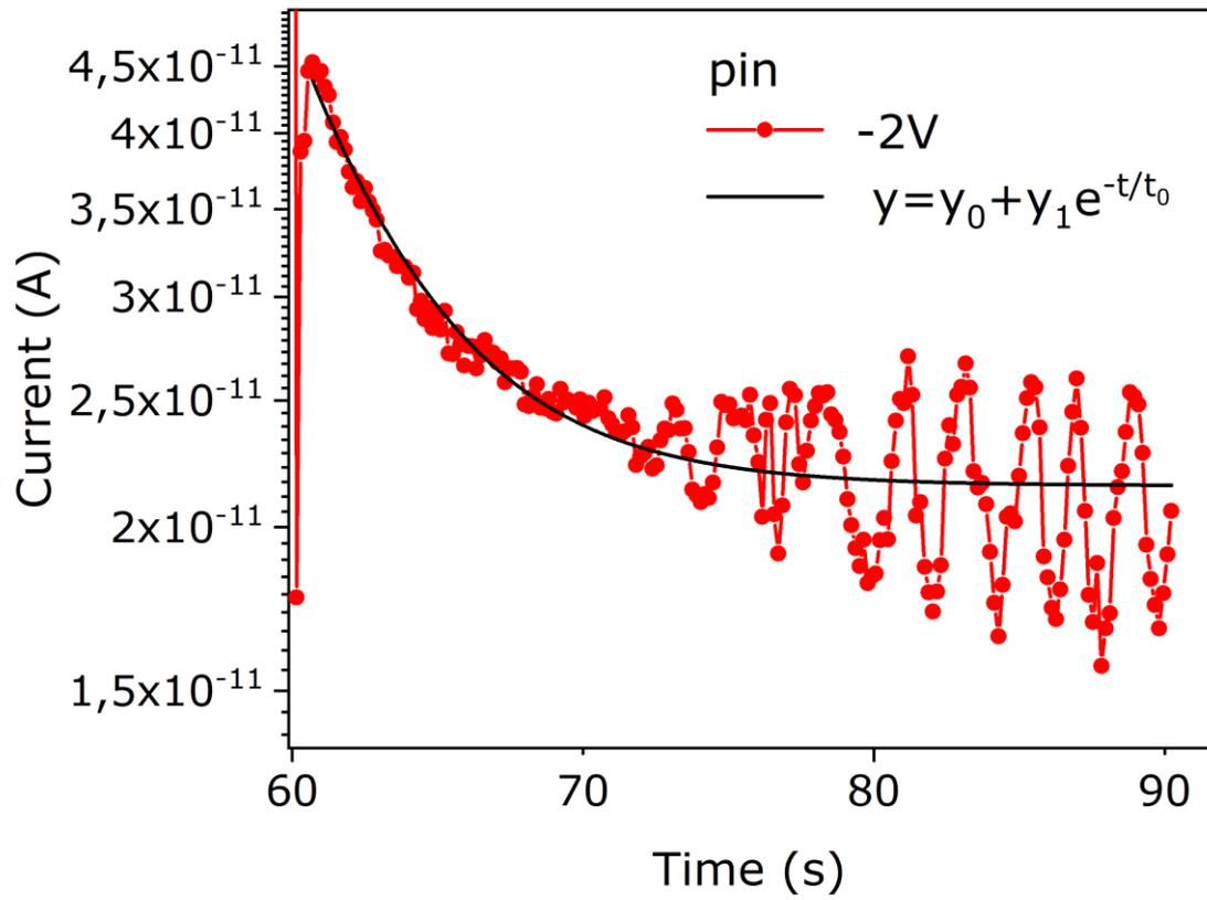
Figure S2: Exponential fit  $y = y_0 + y_1 e^{-t/t_0}$  of the transient time of a pin GaN diode biased at -2V after the ON-OFF transient of 150ms during proton irradiation (64.8MeV, 132pA/cm<sup>2</sup>).
