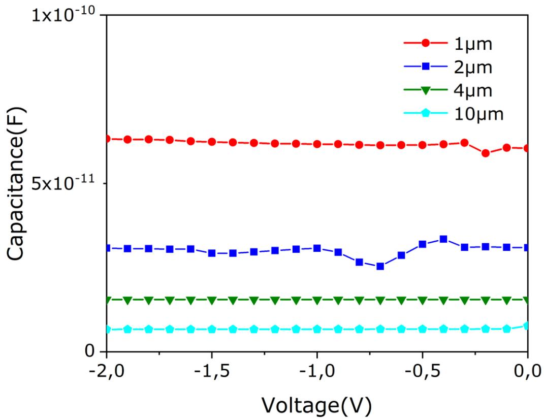
Figure S5: C-V measurement of GaN Schottky diodes on Sapphire at 20kHz, for the samples with different nid layer thicknesses, as reported in the legend. The Capacitance values at 0V are used for the calculation of the depletion layer thickness.
