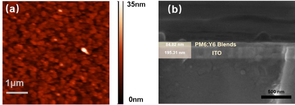
**Fig. S2.** (a) AFM images of blends films with mass ratio of ITO/PM6 : Y6/Au device; (b) SEM image of the section of the device (thickness of active layer is 84.82 nm, thickness of ITO electrode is 195.31 nm).
