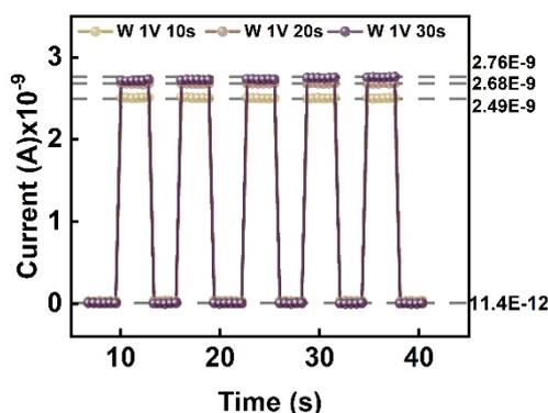
**Fig. S4.** The influence of different bias stimulation times on the photocurrent of the device under the same light intensity and white light
