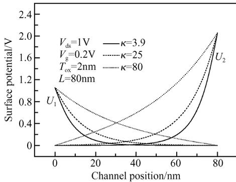
Fig.6 Distribution of surface potential  $U_1(x, y)$  and  $U_2(x, y)$  for different  $k$  values
