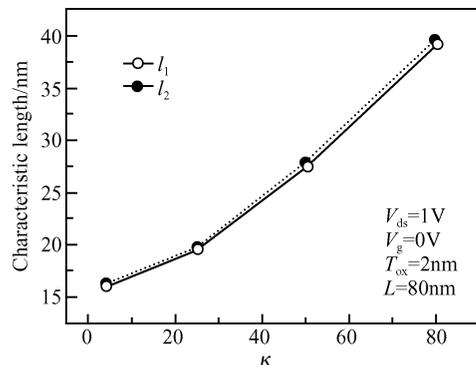
Fig. 9 Changes of the characteristic lengths as a function of  $k$
