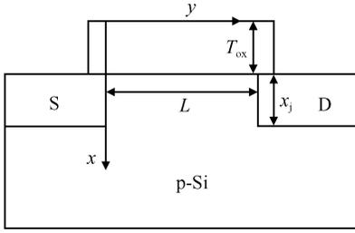
Fig.1 Schematic diagram of nMOSFET structure
