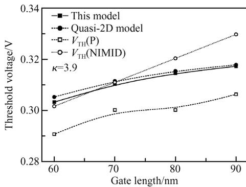
Fig. 3 Comparison between the simulated and experimental threshold voltages
