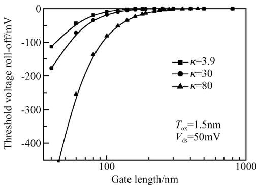
Fig. 7 Dependence of the threshold voltage roll-off on channel length with different gate dielectric constants
