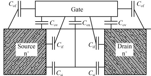
Fig.2 Schematic of the different capacitance components
