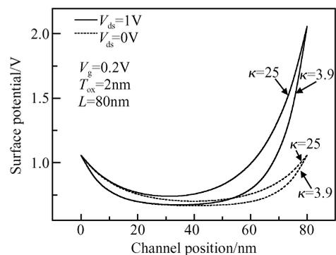
Fig. 5 Surface-potential distribution for different  $\kappa$  and  $V_{ds}$   $x = 0\text{nm}$  and  $80\text{nm}$  are the source and drain ends of the channel, respectively.
