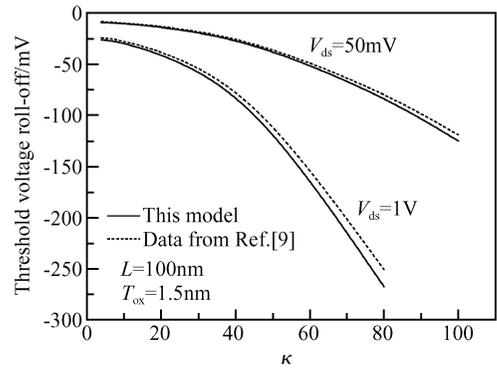
Fig. 4 Threshold voltage roll-off versus gate dielectric constant
