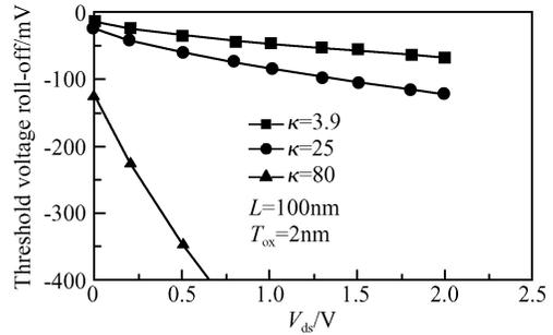
Fig. 8 Dependence of the threshold voltage roll-off on  $V_{ds}$
