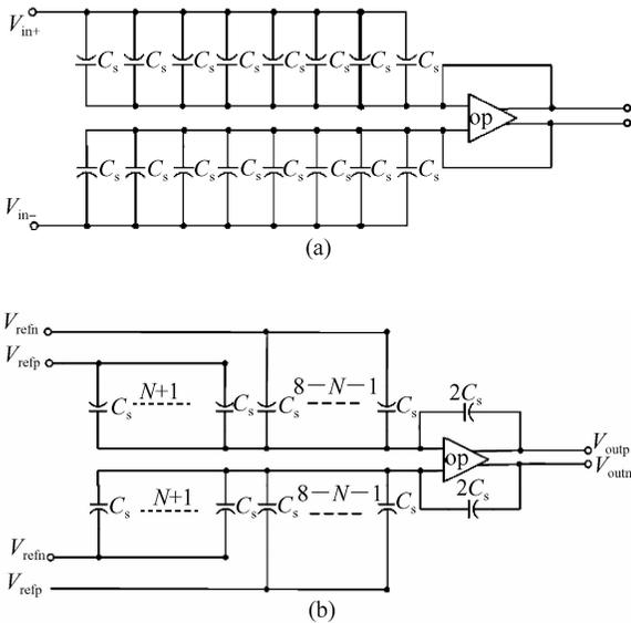
Fig.5 (a) Capacitor array DAC in sampling stage; (b) Capacitor array DAC in generating reference voltage stage
