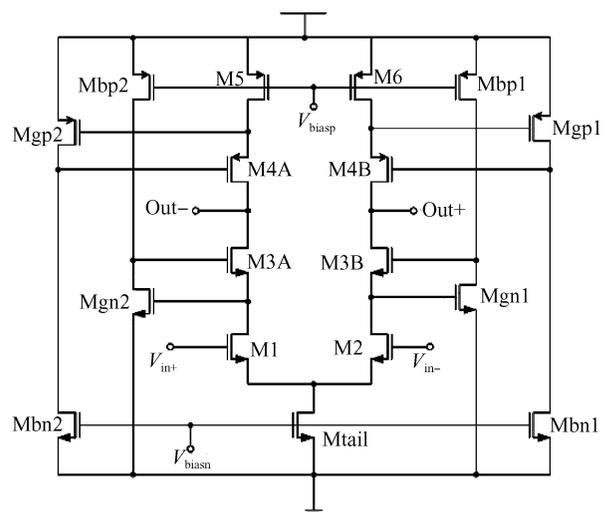
Fig.2 Residue amplifier circuit
