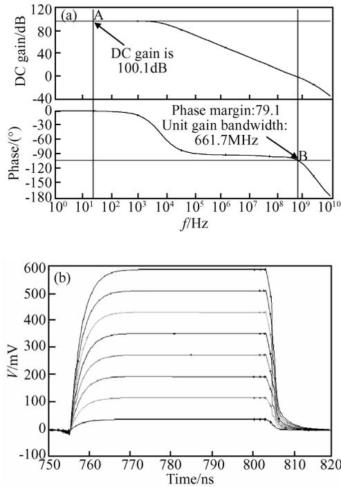
Fig. 3 (a) AC response curve of the amplifier; (b) Transient response of the amplifier
