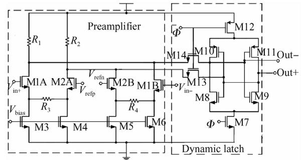
Fig. 4 Comparator circuit
