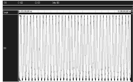
Fig. 8 A 1kHz sine wave recorded by Tektronix TLA5201 logic analyzer
