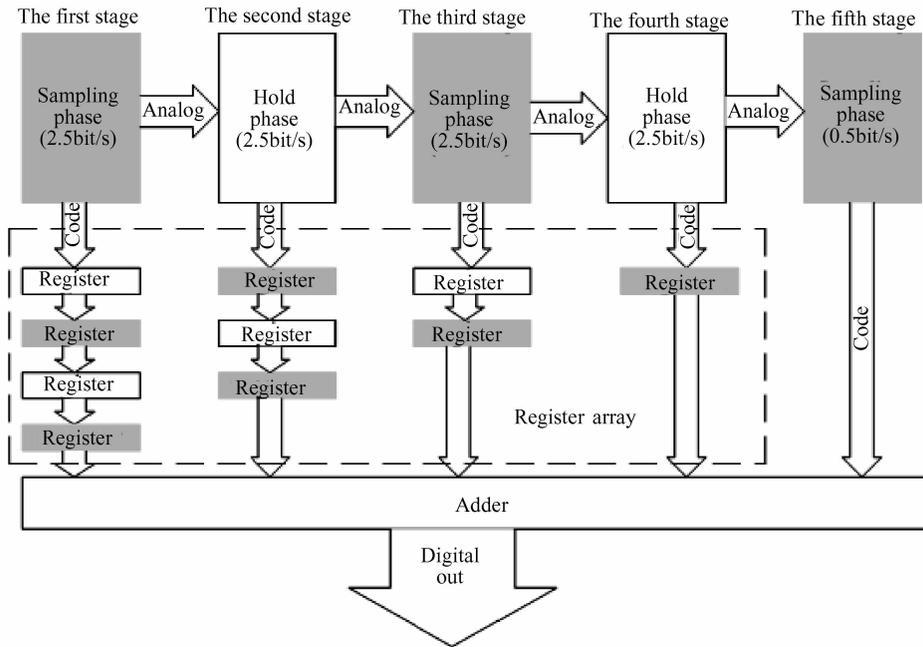
Fig.1 Structure of an ADC system
