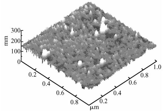
Fig.3 AFM image of ZnO film grown at 300°C
