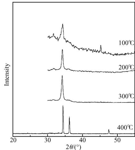
Fig.1 XRD spectra of the ZnO films grown on GaAs substrate at different temperatures
