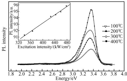
Fig. 4 Normalized PL spectra of ZnO films grown at different temperatures measured at room temperature
