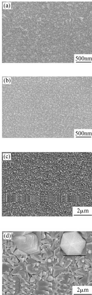
Fig.2 Surface morphology of ZnO films grown at 100°C (a), 200°C (b), 300°C (c), and 400°C (d). The inset images are enlarged images of hexagonal and multi-layer tower structure grains with a bar of 500nm.
