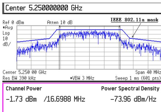
Fig.10. Output spectrum for 64-QAM OFDM modulated signal.
