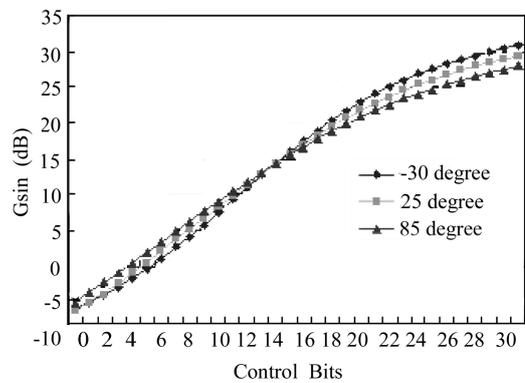
Fig.8. Power gain (dB) versus control bits with varying temperature.
