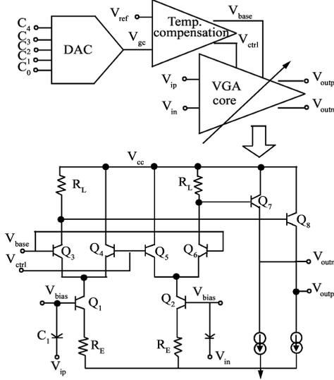
Fig.1. Block diagram of the VGA and the circuit schematic of the VGA core.
