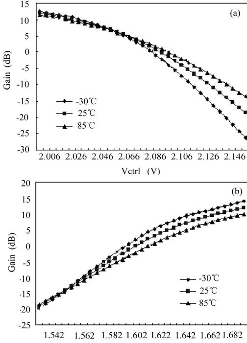
Fig.4. Simulated gain of VGA at the temperature varying from  $-30$  to  $85$  °C: (a) Without temperature compensation; (b) With temperature compensation.
