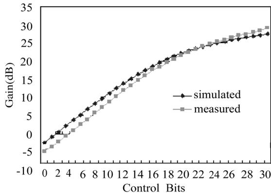
Fig.7. Comparison between the simulated and measured power gain of the VGA and PA driver.
