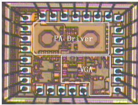
Fig.6. Die photo of the VGA and PA driver.
