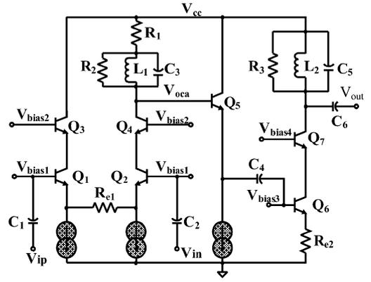
Fig.5. Schematic of the power amplifier driver.
