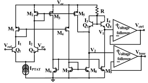
Fig.2. Circuit schematic of the temperature compensation.
