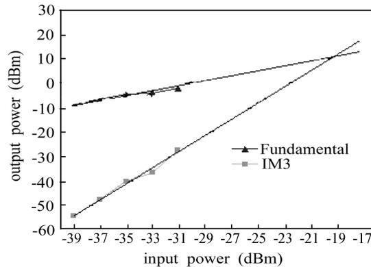
Fig.9. Third-order intermodulation characteristic of the VGA and PA driver.
