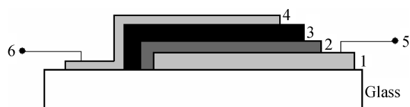
Fig. 1. Cross-sectional view of ITO/CuPc/C 60 /Al cell: 1-ITO, 2-CuPc, 3-C 60 , 4-Al, 5 and 6-terminals.
