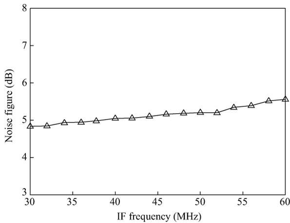
Fig. 8. Measured noise figure of the IF band.
