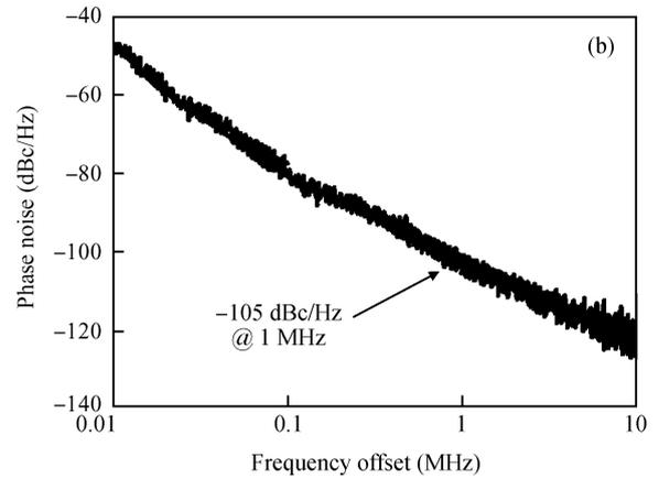
Fig. 10. Phase noise on (a) the VCO test ports of 2.444 GHz and (b) the divider test ports of 1.222 GHz.
