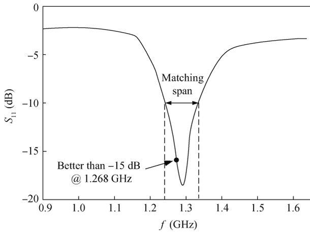
Fig. 7.  $S_{11}$  matching of the transconductance stage.
