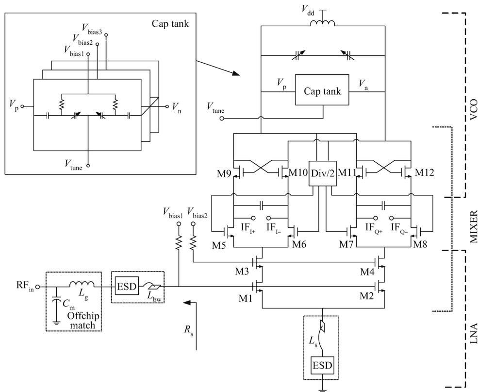
Fig. 1. Schematic of single-inductor quadrature LNA-mixer-VCO.
