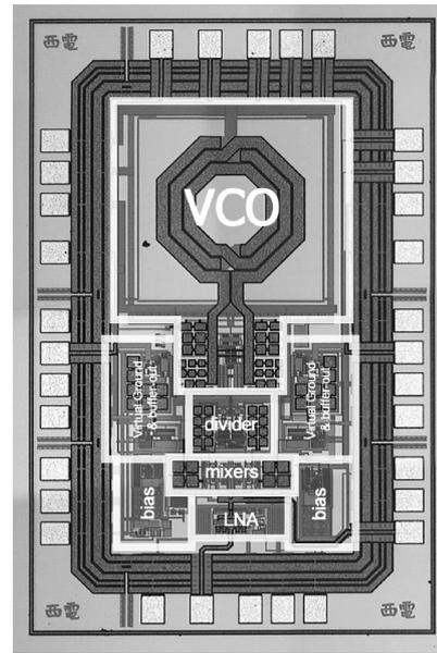
Fig. 5. Micrograph of the test-chip.
