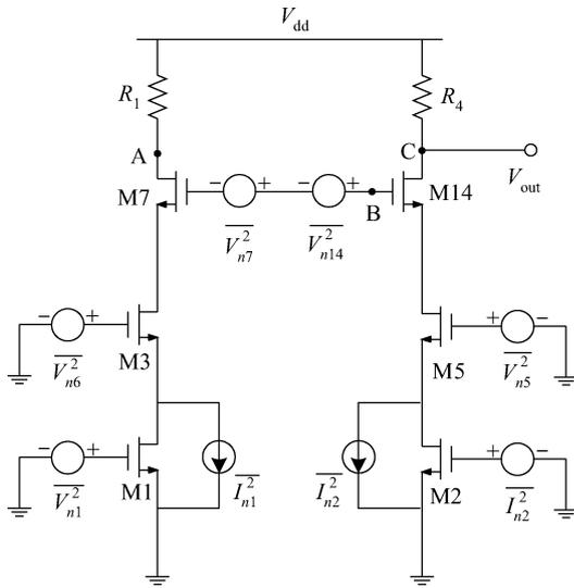
Fig. 4. Simplified schematic of the small signal model of a divider with noise source.
