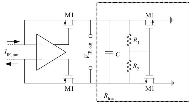
Fig. 3. Low-frequency virtual ground circuit.
