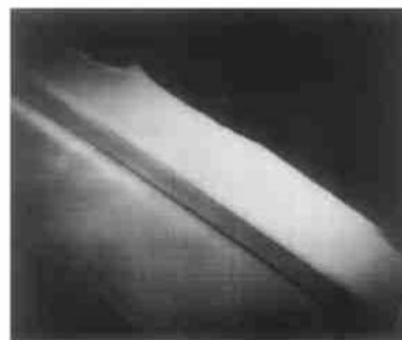
FIG. 2 Cross-Sectional TEM Micrograph of Si/SiGe/Si n-p-n HBT Structure Materials
