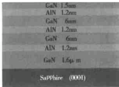
图 2 AlN/GaN 超晶格二维电子气材料结构 Fig. 2 Schematic structure of AlN/GaN superlattice two-dimensional electron gas structure
