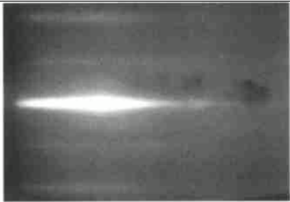
图 1 GaN 膜生长时沿 [\bar{1}120] 方位的 RHEED 图形 Fig. 1 RHEED pattern of GaN thin film along [\bar{1}120] azimuth
