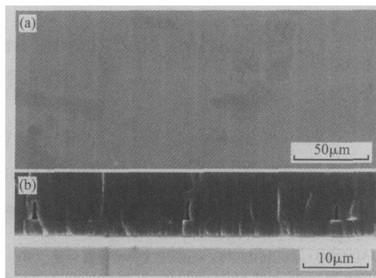
Fig. 1 Plane view (a) and cross-sectional view (b) of SEM images for coalesced ELOG GaN samples. One of the merging front related contrast lines is highlighted by a vertical arrow.
