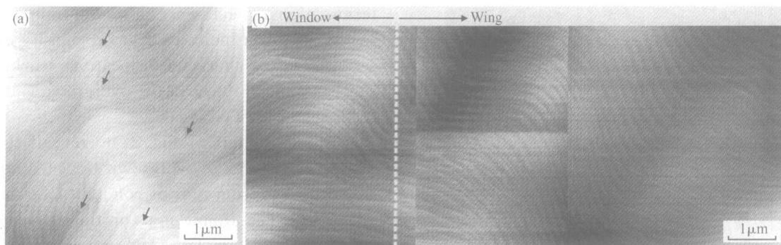
Fig. 3 (a) An AFM image of typical GaN film showing step terminations that are due to the intersection of either a pure screw or mixed threading dislocation with the film surface; (b) Montages of AFM images of successive  $4\mu\text{m} \times 4\mu\text{m}$  scans from window to wing, where dark arrows are shown as a guide to the eye to point out the step terminations
