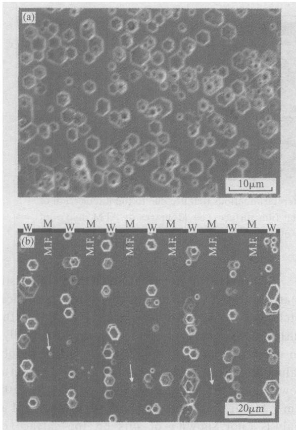
Fig.2 Surface morphology of GaN template (a) and ELOG GaN (b) after etching in molten KOH, where the symbols M, W, and M. F. indicate the region over the mask, window region, and merging front, respectively
