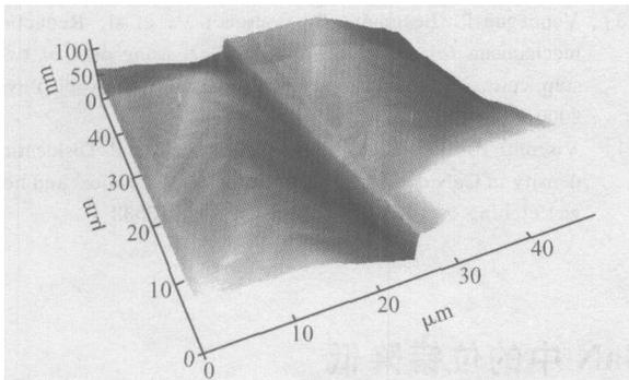
Fig. 5 50μm x50μm AFM scan of ELOG GaN
